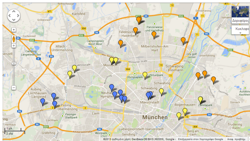
Figure 27: Munich Dataset: Groups created for the furniture delivery scenario. Each customer is represented by a marker. In this case, customers are divided into 3 groups, served by two vehicles that perform three tours.
