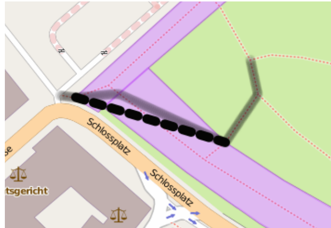
Figure 3.12: An example for touching areas that need to be merged, before they can be properly traversed via visibility graph edges.
