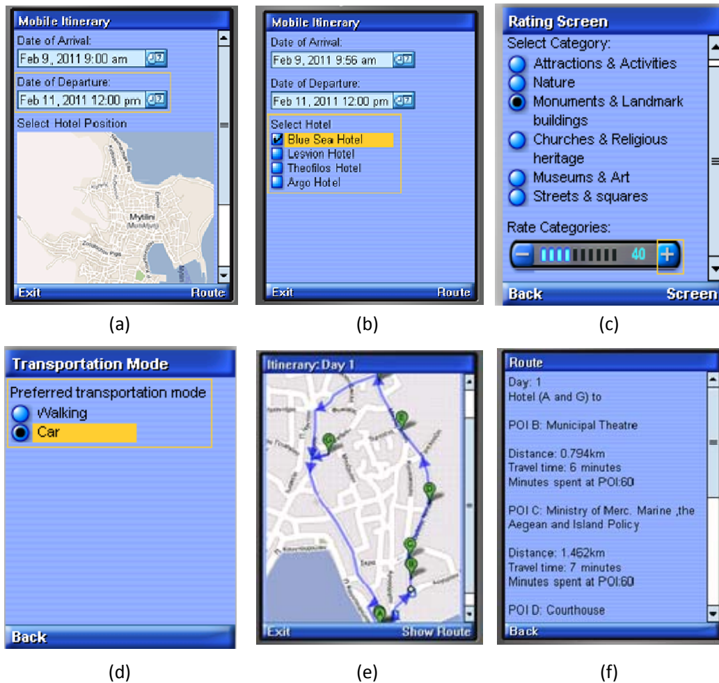
Figure 4. Screens of the DailyTRIP mobile web application: (a) accommodation’s selection through a map interface; (b) accommodations’ selection through a set of predefined choices; (c) rating of POI categories (0-100 scale, with step 20); (d) selection of preferred transportation mode; (e) visualization of a daily itinerary; (f) textual description of a daily itinerary.
